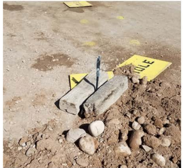
The Inzwa Veva III allows for flexible antenna solutions. Here an extended antenna was used to allow the device to be buried and still access the available cell service.
