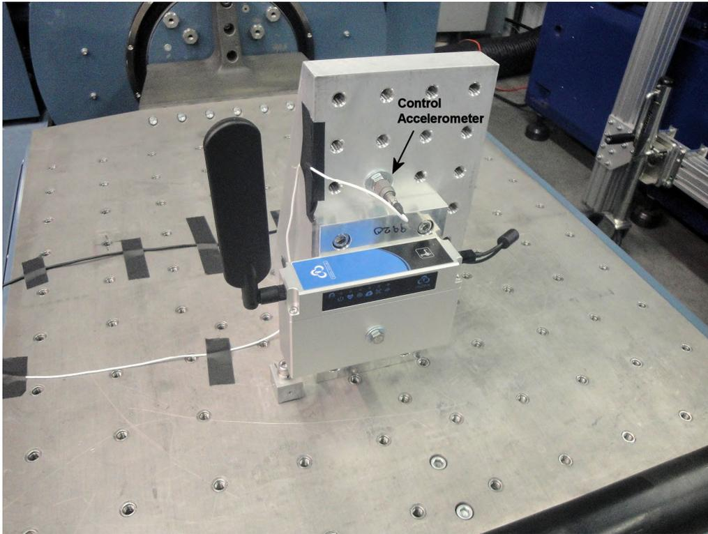
**Figure 1.2.2 Y Axis Setup (Control from Angle)**
