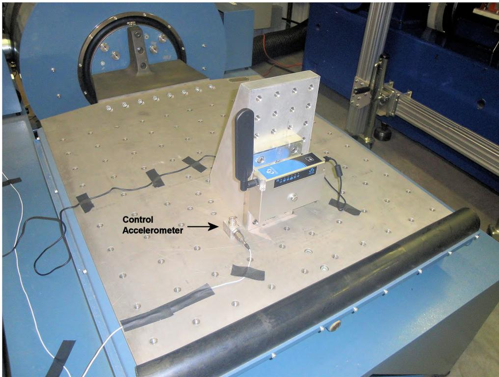
**Figure 1.2.1 Y Axis Setup (Control from Slip Table)**
