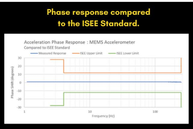
A prototype MEMS accelerometer was then developed and placed in field trials against two of the industry's widely accepted seismographs known for compliance with ISEE standards. A total of 55 events were monitored with resultant PPV values ranging from 0.8 mm/s (0.03 i.p.s) to 58.5 mm/s (2.3 i.p.s). **Resultant PPV values from the standard seismographs plotted against that recorded with the accelerometer-based prototype showed correlation coefficient between the data sets is 0.992.**
